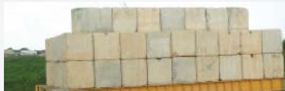
Concrete blocks used in static pile load test (Kentledge method).
